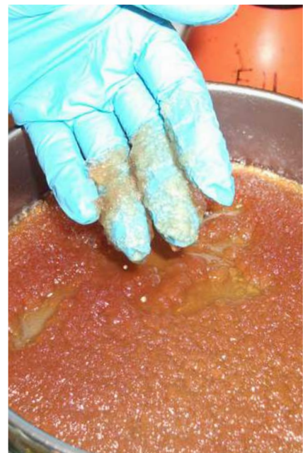
Fig. 13: Waxy precipitations in a fuel sample
